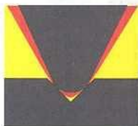
COMPARISON OF CONVENTIONAL ELLIPTICAL STYLUS (BLACK) TO SHIBATA-TYPE STYLUS (RED). SHIBATA-TYPE STYLUS TRACES MORE OF THE GROOVE INFORMATION AND PLACES LESS TENSION UPON THE DISC SURFACE.
